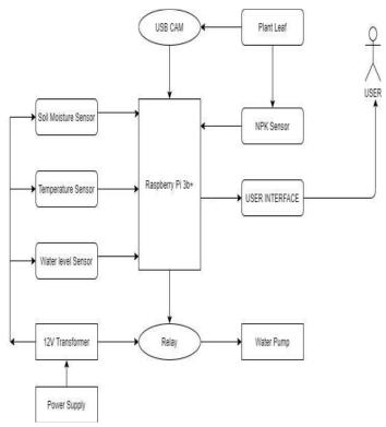
Figure 1: Block Diagram of Working Model.
